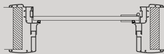
Anta interamente in laminato stratificato sp. 14mm / door entirely in 14 mm thick stratified laminate
